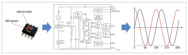
Compensation of the temperature coefficient leads to a high output voltage over the full temperature range. This in turn leads to a high signal resolution at the microcontroller ADC. The temperature-dependent output voltage at pin VTEMP
