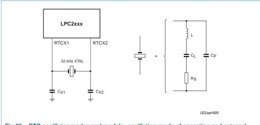
Fig 23. RTC oscillator modes and models: oscillation mode of operation and external crystal model used for  $C_{X1}/C_{X2}$  evaluation
