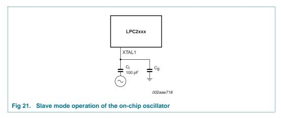
In slave mode the input clock signal should be coupled by means of a capacitor of 100 pF (Figure 21), with an amplitude between 200 mV (RMS) and 1000 mV (RMS). This corresponds to a square wave signal with a signal swing of between 280 mV and 1.4 V. The XTALOUT pin in this configuration can be left unconnected.
