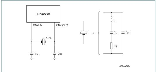
Fig 22. Oscillator modes and models: oscillation mode of operation and external crystal model used for  $C_{X1}/C_{X2}$  evaluation
