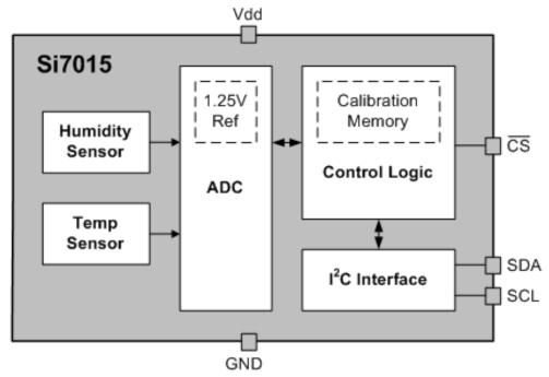
Figure 5. Si7015 Functional Block Diagram
