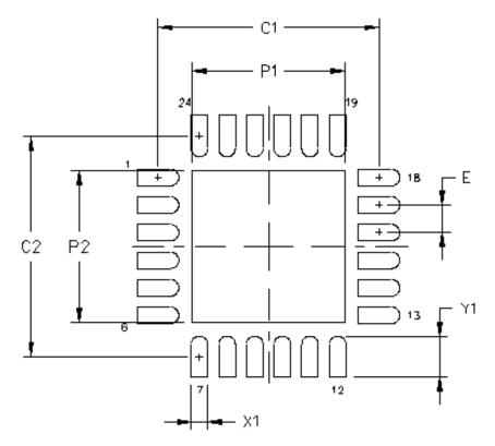
Figure 10. Typical QFN-24 PCB Land Pattern
