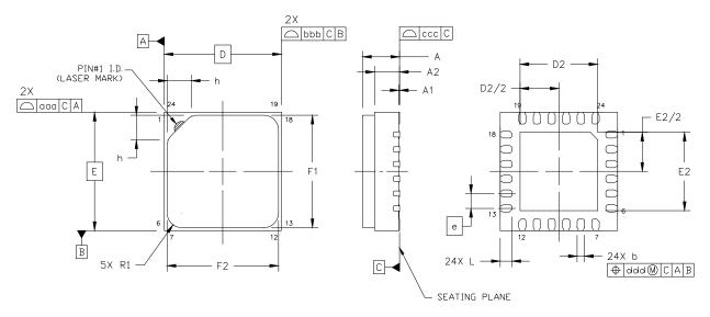
Figure 9. 24-Pin Quad Flat No Lead (QFN) With Protective Cover
