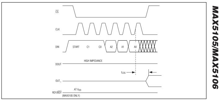
Figure 8. Nonvolatile Load Command Timing Diagram
