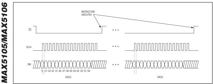
Figure 2. 3-Wire Interface Timing
