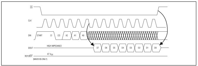
Figure 7. Nonvolatile Read Command Timing Diagram
