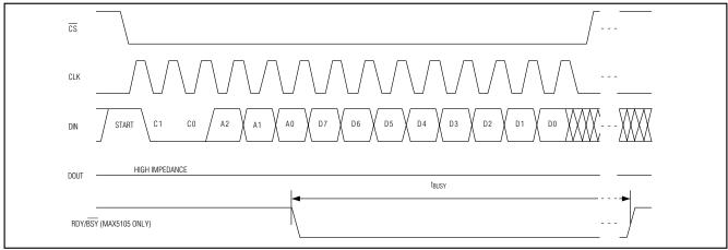
Figure 5. Nonvolatile Store Command Timing Diagram
