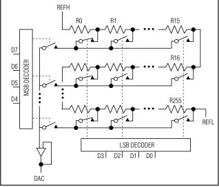
Figure 1. DAC Simplified Circuit Diagram
