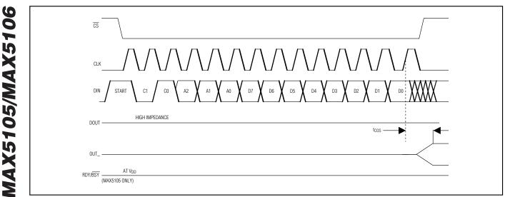
Figure 6. Register Write Command Timing Diagram
