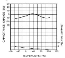
Fig.3 Capacitance - temperature characteristics
