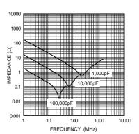
Fig.4 Impedance - frequency characteristics
