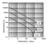
Fig.2 Impedance - frequency characteristics
