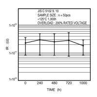
Fig.21 Insulation resistance
