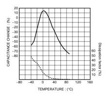
Fig.5 Capacitance - temperature characteristics
