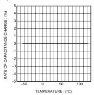
Fig.1 Capacitance - temperature characteristics
