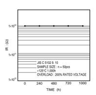
Fig.18 Insulation resistance
