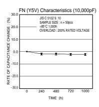
Fig.22 Rate of capacitance change
