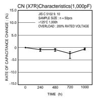
Fig.19 Rate of capacitance change
