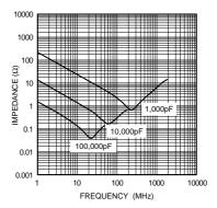
Fig.6 Impedance - frequency characteristics
