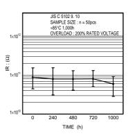
Fig.24 Insulation resistance
