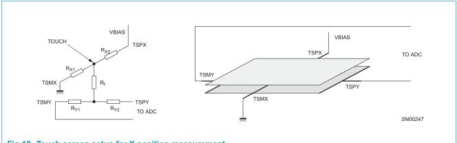
Fig 18. Touch screen setup for X position measurement.
