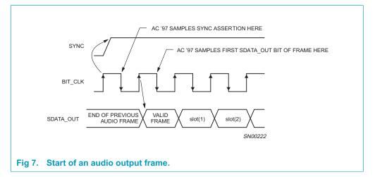
SDAT\_OUT's composite stream is MSB justified (MSB first) with all non-valid slots' bit positions stuffed with 0s by the AC '97 Controller. If there are less than 20 valid bits within an assigned and valid time slot, the AC '97 Controller always stuffs all trailing non-valid bit positions of the 20-bit slot with 0s.
