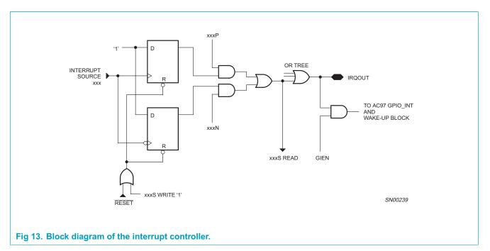
The interrupt generation mode is set by the Positive INT Enable Register (0x5E) and Negative INT Enable Register (0x60). The actual interrupt status of each signal can be read from the INT Clear/Status Register (0x62). The interrupt status is cleared whenever a '1' is written in the INT Clear/Status Register (0x62) for the corresponding bit.
