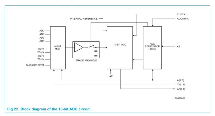
The ADC is controlled through the AC '97 interface, but the UCB1400 contains internal logic to ease the control of the ADC and to minimize the number of AC '97 frame read/write actions.
