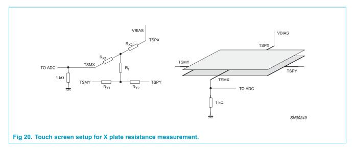
The plate resistance of a touch screen varies a lot due to processing spreads. Knowing the actual plate resistance makes it possible to compensate for the plate resistance effects in the pressure resistance measurements. Secondly, the plate resistance decreases when two or more spots on the touch screen are pressed. In that case, a part of one plate, e.g., the X plate, is shorted by the other plate, which decreases the actual plate resistance.
