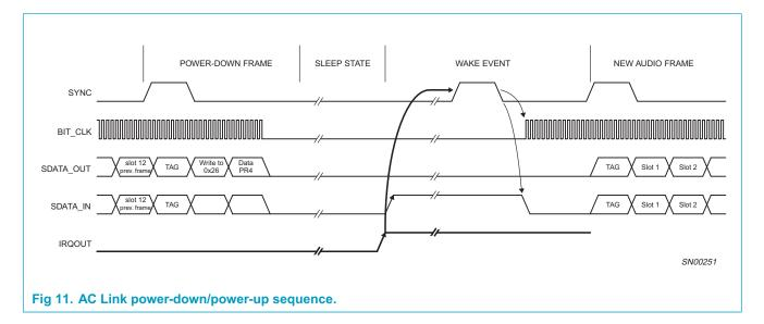
Before enabling wake-up via IRQOUT or GIEN bit, the UCB1400 must be enabled for interrupt by setting the appropriate bits in the Positive INT Enable register (0x5E) and Negative INT Enable register (0x60). The INT Clear/Status register (0x62) should then be cleared of any previous interrupts before going to low-power mode.
