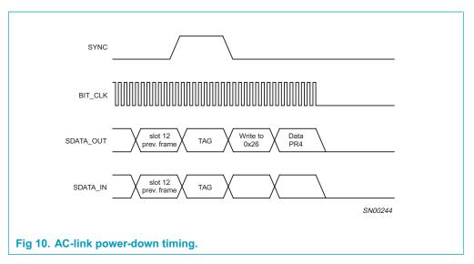
BIT\_CLK and SDATA\_IN are transitioned low immediately following the decode of the write to Register 0x26 with PR4. When the AC '97 Controller driver is at the point where it is ready to program the AC-link into its low power mode, slots (1 and 2) **are assumed to be** the only valid stream in the audio output frame.
