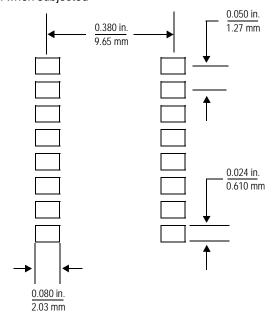
Figure 6. Footprint SOIC-16 (Case 475-01)
