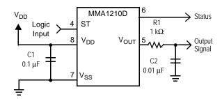
Figure 4. SOIC Accelerometer with Recommended Connection Diagram
