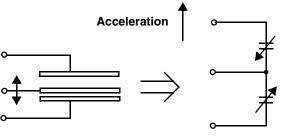
Figure 2. Transducer Physical Model
