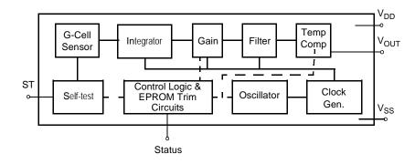
Figure 1. Simplified Accelerometer Functional Block Diagram
