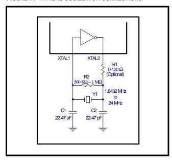
FIGURE 7. TYPICAL OSCILLATOR CONNECTIONS
