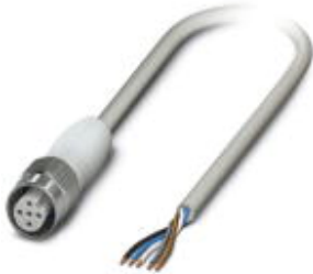
Sensor/Actuator cable, 5-position, PP-EPDM halogen-free, Gray RAL 7035, Free cable end, on Socket straight M12, A-coded, Cable length: 5 m, Hygienic design, With high-grade steel knurl
