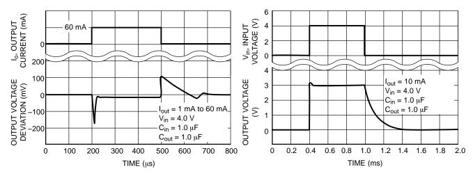
Figure 10. Load Transient Response
