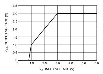
Figure 12. Output Voltage vs. Input Voltage
