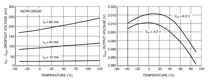
Figure 2. Dropout Voltage vs. Temperature
