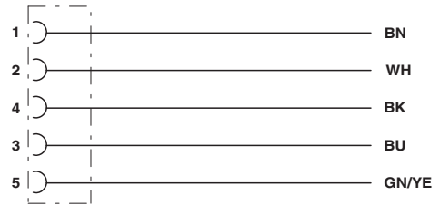
Contact assignment of the M12 socket
