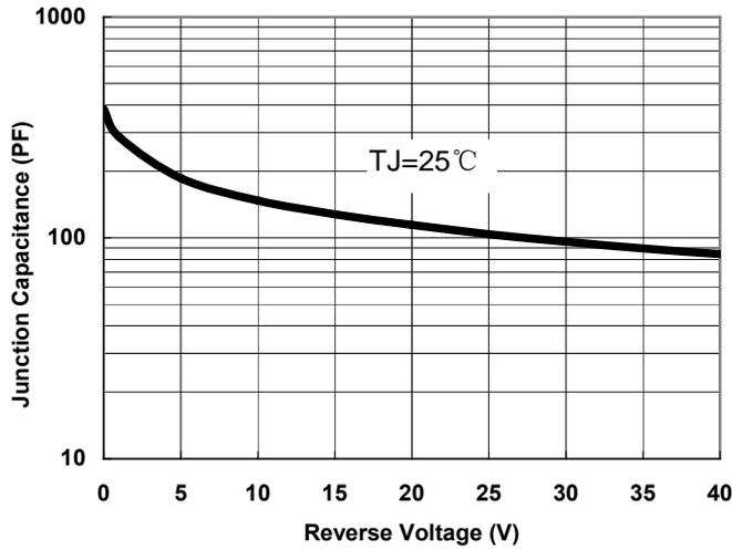
Fig.1-Typical Junction Capacitance
