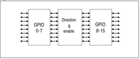
When enabled, the GPIO 0-7 bits are internally mapped to GPIO 8-15 bits. The STMPE1601 becomes an 8-channel level translator where each of the channels may have its direction set individually. As GPIO 0-7 operates from Vcc, and GPIO 8-15 operates from  $V_{IO}$ , this allows the 2 groups of GPIOs to work as a level translator.
