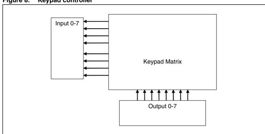
Figure 8. Keypad controller
