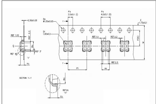
Figure 12. Carrier tape information for TFBGA25
