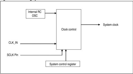
The decision on clocks is based on the bits written into the SYS\_CTRL registers. Bits 0 to 3 of the SYS\_CTRL register allow to control the gating of clocks to the keypad controller, PWM and GPIO in the operational mode.
