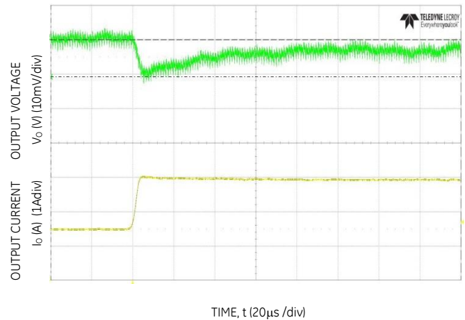
Figure 10. Transient Response to Dynamic Load Change from 50% to 100% at 12Vin, C out =6x47µF+1x330µF, C Tune =5600pF, R Tune =300Ω
