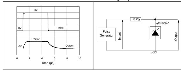
Figure 9. Pulse response for  $I_k=1$ mA
