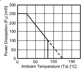
Figure 3 Power Dissipation of Package
