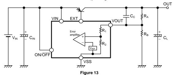
The S-816 Series has an internal impedance resulting from  $R_1$  and  $R_2$  between the VOUT and the VSS pin, as shown in **Figure 13**. Therefore, the influence of the internal resistances ( $R_1$ ,  $R_2$ ) of the IC has to be taken into consideration in defining the output voltage (OUT).
