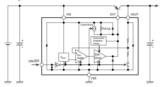
**Remark 1.** To ensure you power cutoff of the external transistor when the device is powered down, the EXT output is pulled up to  $V_{IN}$  by a pull-up resistance (approx. 0.5  $M\Omega$ ) inside the IC.
