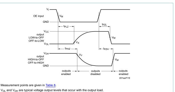
Fig 11. Enable and disable times
