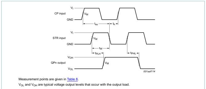
Fig 9. Propagation delay strobe input (STR) to output (QPn), strobe input (STR) pulse width and the clock set-up and hold times for strobe input
