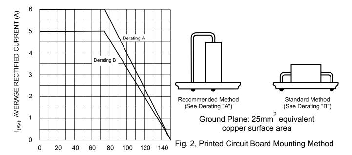
T<sub>A</sub>, AMBIENT TEMPERATURE (°C) Fig. 1, Forward Current Derating Curve
