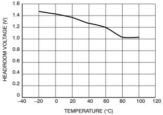
Figure 6. Headroom versus Temperature
