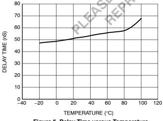
Figure 5. Delay Time versus Temperature
