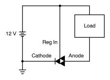
Figure 11. Negative ORing Diode Connection
