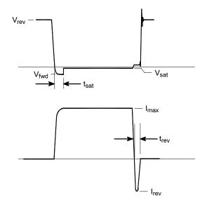
Figure 1. Switching Waveform
