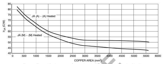
Figure 7. Thermal Resistance vs. Copper Area for MOSFET (M) and Analog Die (A)
