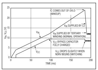
Figure 2. VIN and VCC During Startup
