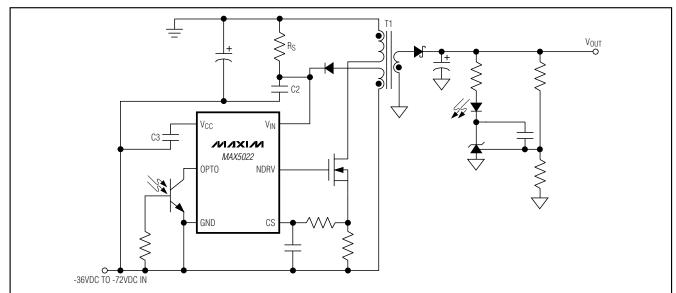
Figure 4. -48VDC Input to +5V Output
