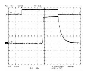
FIGURE 12. ENABLE FUNCTION (V  $_{IN}$  = 3.6V, V  $_{OUT}$  = 1.85V, C  $_{OUT}$  1 $\mu F$ )
