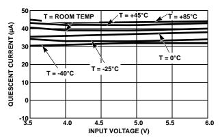
FIGURE 3. QUIESCENT CURRENT vs INPUT VOLTAGE  $(V_{OUT} = 3.3V)$
