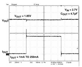
FIGURE 11. LOAD TRANSIENT RESPONSE
