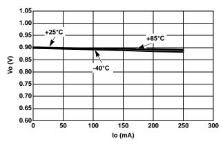
FIGURE 8. LOAD REGULATION vs TEMPERATURE  $(V_{OUT} = 0.9V)$
