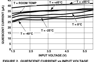
FIGURE 2. QUIESCENT CURRENT vs INPUT VOLTAGE (V<sub>OUT</sub> = 1.85V)
