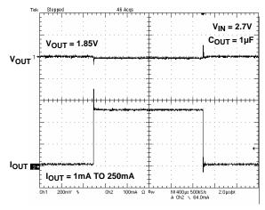
FIGURE 10. LOAD TRANSIENT RESPONSE
