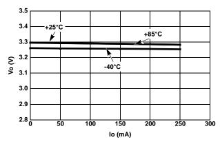
FIGURE 6. LOAD REGULATION vs TEMPERATURE  $(V_{OUT} = 3.3V)$
