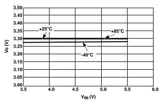
FIGURE 7. LINE REGULATION vs TEMPERATURE  $(V_{OUT} = 3.3V)$
