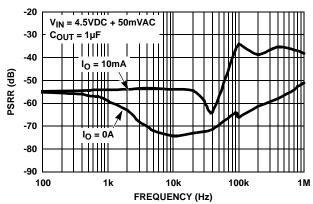
FIGURE 13. POWER SUPPLY REJECTION vs FREQUENCY
