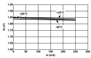
FIGURE 4. LOAD REGULATION vs TEMPERATURE (V<sub>OUT</sub> = 1.85V)
