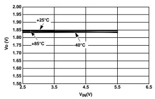
FIGURE 5. LINE REGULATION vs TEMPERATURE (V<sub>OUT</sub> = 1.85V)
