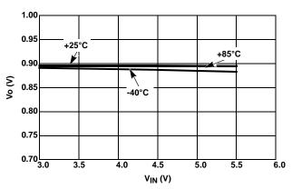
FIGURE 9. LINE REGULATION vs TEMPERATURE  $(V_{OUT} = 0.9V)$
