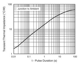
Fig. 6 - Typical Transient Thermal Impedance
