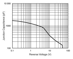
Fig. 5 - Typical Junction Capacitance
