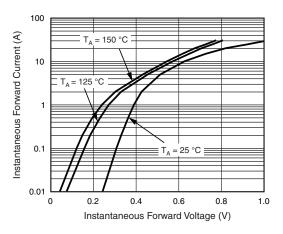
Fig. 3 - Typical Instantaneous Forward Characteristics
