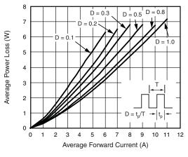
Fig. 2 - Forward Power Loss Characteristics
