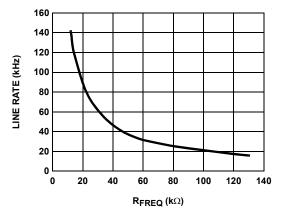
FIGURE 22. LINE RATE vs RFREQ
