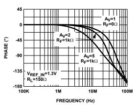
FIGURE 2. NON-INVERTING FREQUENCY RESPONSE (PHASE)
