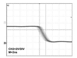
FIGURE 39. JITTER AT THE OUTPUTS WITH FSEL=1
