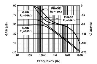
FIGURE 9. OPEN LOOP GAIN AND PHASE vs FREQUENCY
