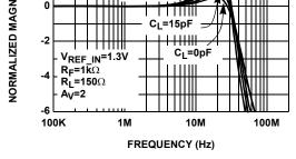
FIGURE 7. FREQUENCY RESPONSE FOR VARIOUS CL
