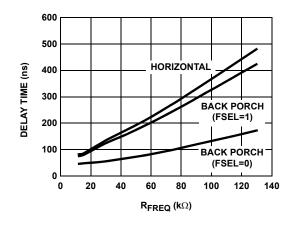
FIGURE 25. DELAY TIME vs RFREQ
