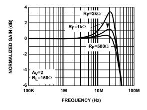
FIGURE 5. FREQUENCY RESPONSE FOR VARIOUS RF
