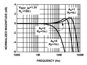
FIGURE 1. NON-INVERTING FREQUENCY RESPONSE (GAIN)
