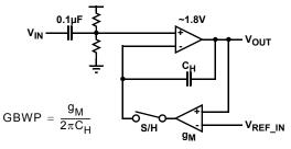
FIGURE 36. DC-RESTORE AMPLIFIER AND S/H CONFIGURATION
