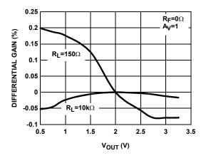
FIGURE 12. DIFFERENTIAL GAIN FOR RL TIED TO 0V
