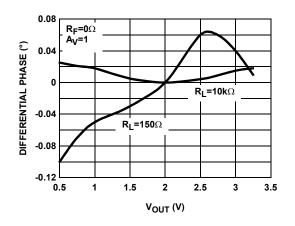
FIGURE 13. DIFFERENTIAL PHASE FOR RL TIED TO 0V
