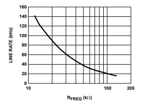
FIGURE 23. LINE RATE vs RFREQ
