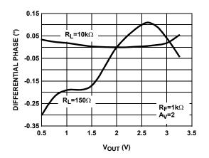
FIGURE 15. DIFFERENTIAL PHASE FOR RL TIED TO 0V
