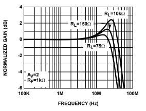
FIGURE 6. FREQUENCY RESPONSE FOR VARIOUS RL
