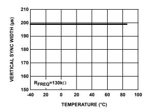
FIGURE 33. VERTICAL SYNC WIDTH vs TEMPERATURE
