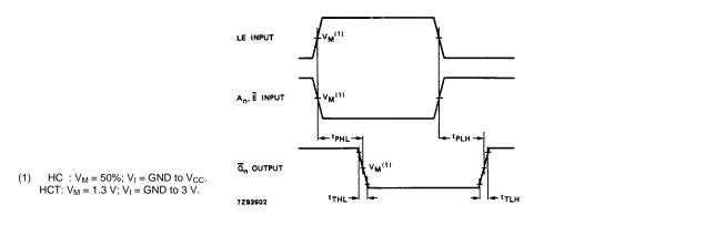
Fig.6 Waveforms showing the input  $(A_n, LE, \overline{E})$  to output  $(\overline{Q}_n)$  propagation delays and the output transition times.
