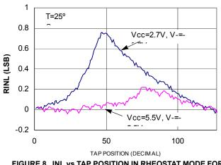
FIGURE 8. INL vs TAP POSITION IN RHEOSTAT MODE FOR 10 k  $\Omega$  (W)
