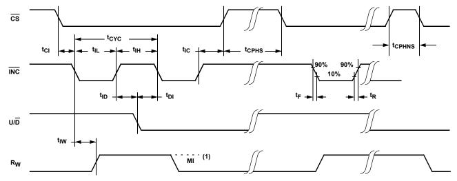
NOTE (1): MI IN THE TIMING DIAGRAM REFERS TO THE MINIMUM INCREMENTAL CHANGE IN THE WIPER POSITION.
