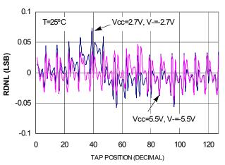
FIGURE 7. DNL vs TAP POSITION IN RHEOSTAT MODE FOR 10k $\Omega$  (W)
