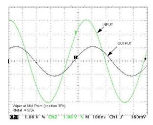
FIGURE 12. FREQUENCY RESPONSE (1.8MHz)
