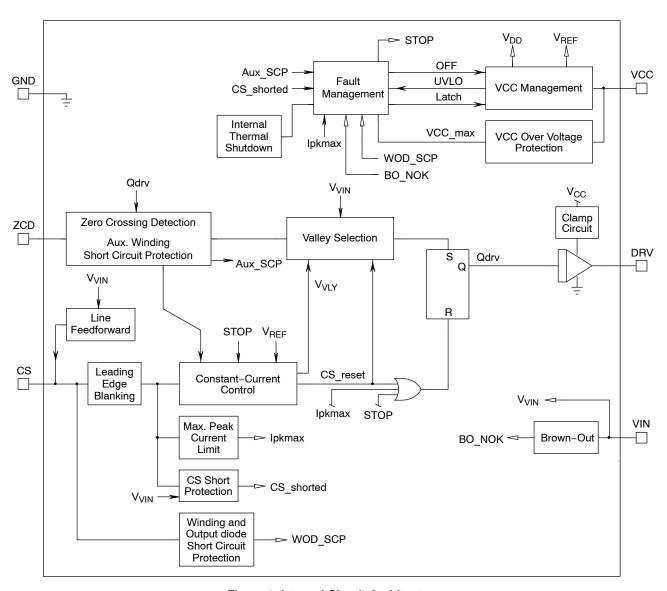
Figure 2. Internal Circuit Architecture
