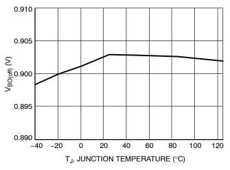
Figure 23.  $V_{BO(off)}$  vs. Junction Temperature
