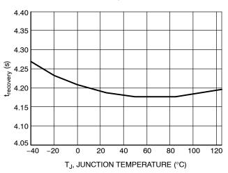
Figure 26.  $t_{recovery}$  vs. Junction Temperature
