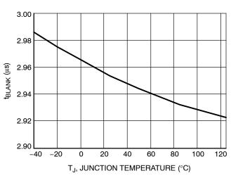
Figure 14. t<sub>BLANK</sub> vs. Junction Temperature
