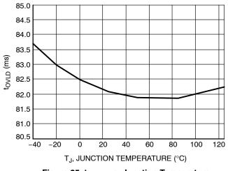
Figure 25. t<sub>OVLD</sub> vs. Junction Temperature
