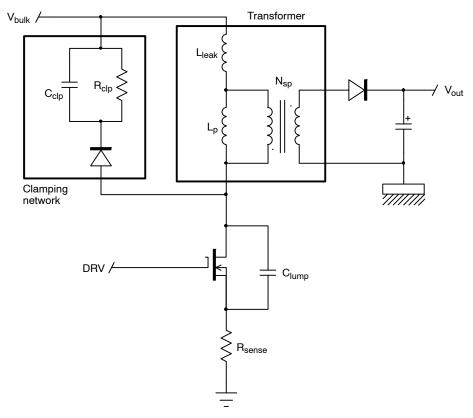
Figure 27. Basic Flyback Converter Schematic
