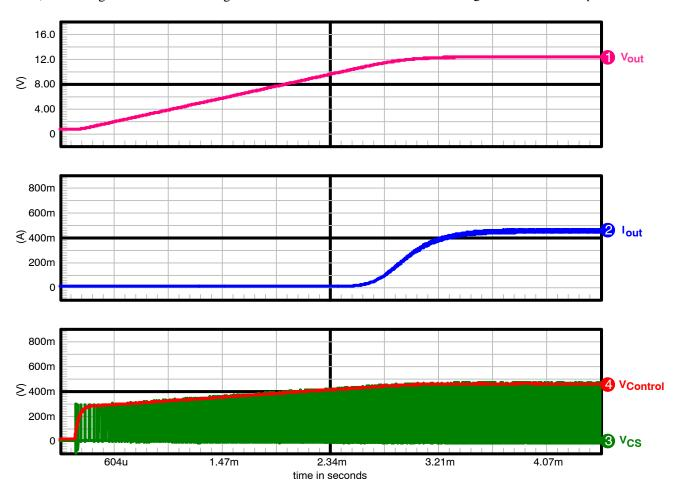
Figure 29. Startup Simulation Showing the Natural Soft-start
