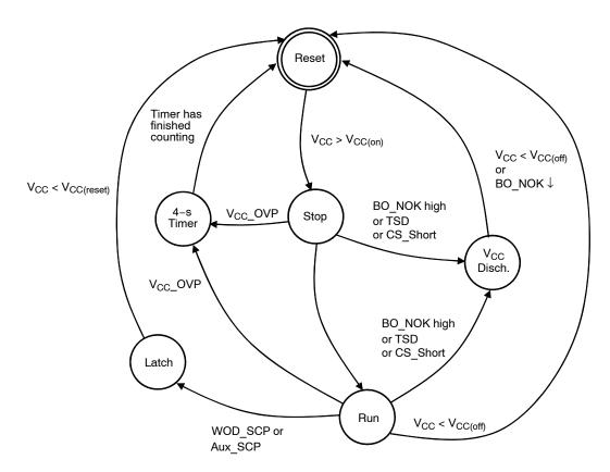
Figure 39. State Diagram for A Version Faults
