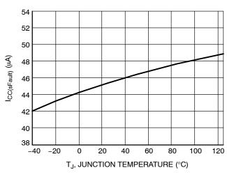
Figure 10. I<sub>CC(sFault)</sub> vs. Junction Temperature
