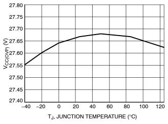
Figure 5. V<sub>CC(OVP)</sub> vs. Junction Temperature
