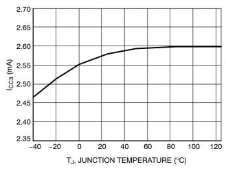
Figure 8. I<sub>CC3</sub> vs. Junction Temperature
