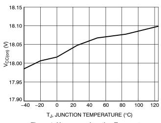
Figure 3.  $V_{CC(on)}$  vs. Junction Temperature
