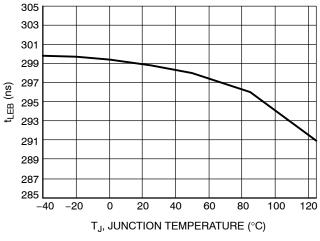
Figure 13. t<sub>LEB</sub> vs. Junction Temperature
