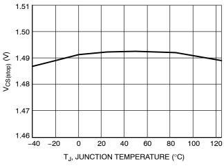
Figure 11. V<sub>CS(stop)</sub> vs. Junction Temperature
