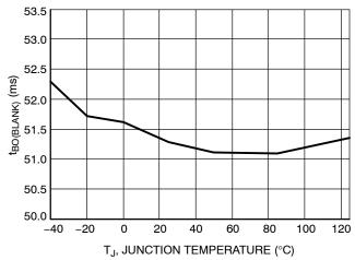
Figure 24. t<sub>BO(BLANK)</sub> vs. Junction Temperature
