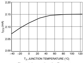
Figure 7. I<sub>CC2</sub> vs. Junction Temperature
