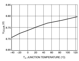
Figure 4. V<sub>CC(off)</sub> vs. Junction Temperature
