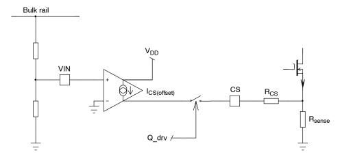
Figure 34. Line Feed-forward Schematic
