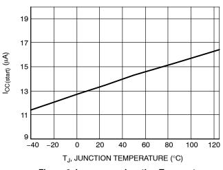
Figure 9. I<sub>CC(start)</sub> vs. Junction Temperature
