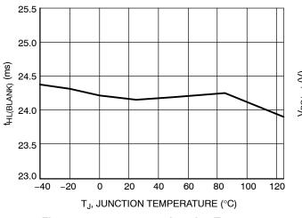
Figure 21. t<sub>HL(BLANK)</sub> vs. Junction Temperature
