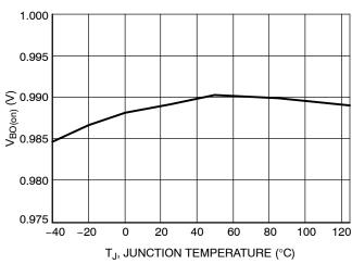
Figure 22.  $V_{BO(on)}$  vs. Junction Temperature
