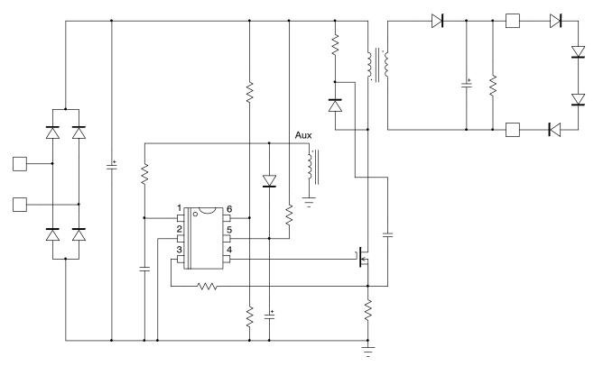
Figure 1. Typical Application Schematic for NCL30080
