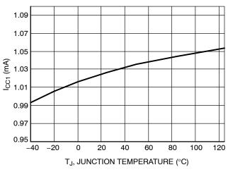
Figure 6. I<sub>CC1</sub> vs. Junction Temperature
