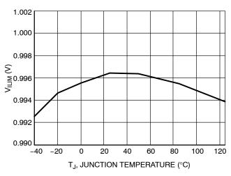
Figure 12. V<sub>ILIM</sub> vs. Junction Temperature
