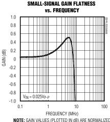
**NOTE:** GAIN VALUES (PLOTTED IN dB) ARE NORMALIZED VALUES RELATIVE TO THE EXPECTED VALUE OF 4V/V.
