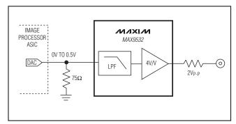
Figure 4. Video DAC Generates a  $0.5V_{P-P}$  Signal Across a  $75\Omega$  Resistor Connected to Ground
