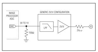
Figure 3. Typically, a Video DAC Generates a  $1V_{P-P}$  Signal Across a  $150\Omega$  Resistor Connected to Ground
