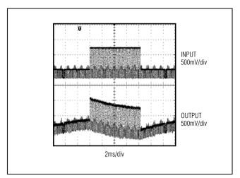
Figure 1. AC-Coupled Output
