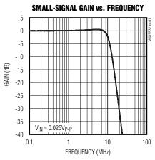
**NOTE:** GAIN VALUES (PLOTTED IN dB) ARE NORMALIZED VALUES RELATIVE TO THE EXPECTED VALUE OF 4V/V.
