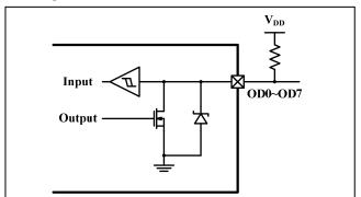
Figure 9 IS31IO7325 Open-Drain I/O Ports Structure
