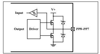
Figure 8 IS31IO7325 Push-Pull I/O Ports Structure
