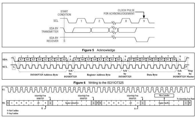
Figure 7 Reading I/O Ports of IS31IO7325
