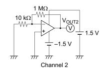
$$CS = \left| 20log_{10} \frac{101 \times |V_{OUT2}|}{|V_{OUT1}|} \right|$$
