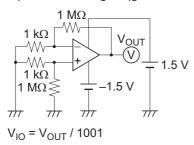
8. Common Mode Input Voltage Range,  $V_{CM}$
