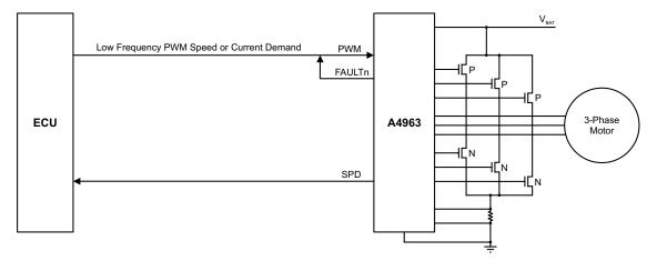
Figure 10: Remote Single-Wire Command with Integrated Closed-Loop Control
