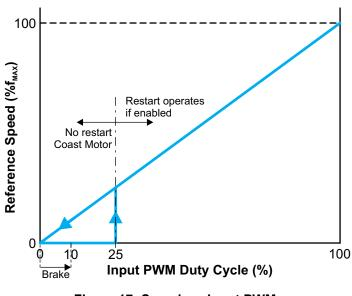
Figure 17: Speed vs. Input PWM
