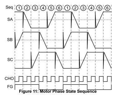
In the A4963, motor speed is always defined as the frequency of the electrical cycle,  $f_{\rm S}$ . This is the same frequency as the FG signal, if selected, on the SPD output.
