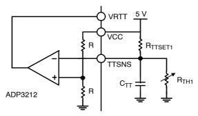
Figure 33. Single–Point Thermal Monitoring
