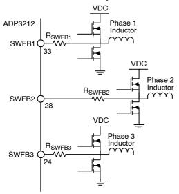
Figure 19. Current Balance Resistors
