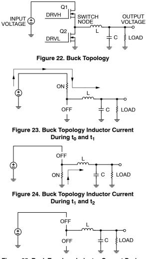
Figure 25. Buck Topology Inductor Current During  $$t_2$ and $t_3$$
