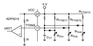
Figure 34. Multiple-Point Thermal Monitoring
