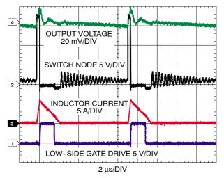
Figure 27. Single-Phase Waveforms in DCM with 1 A Load Current
