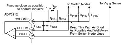
Figure 30. Temperature-Compensation Circuit Values
