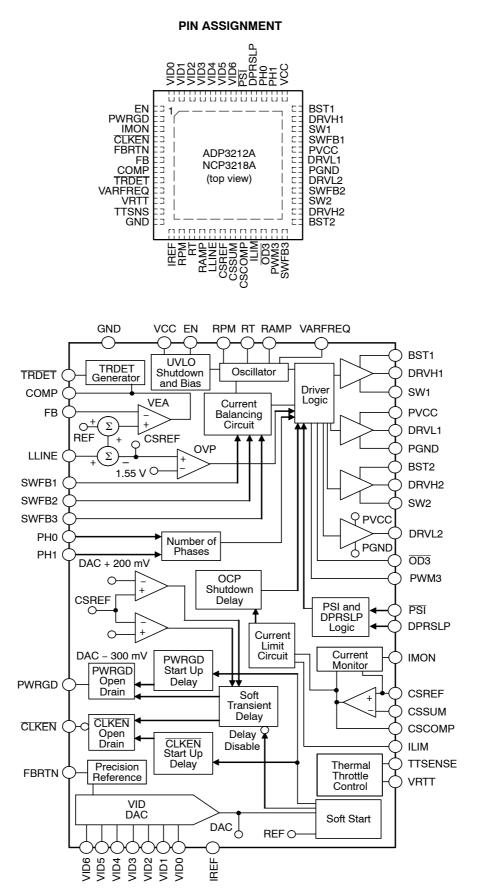
Figure 1. Functional Block Diagram
