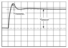
Figure 37. Transient Setting Waveform, Load Release
