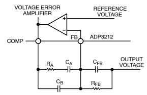
Figure 31. Voltage Error Amplifier
