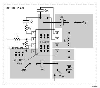
Figure 2. Recommended Component Placement for Boost Converter. Note Direct High Current Paths Using Wide PC Traces. Minimize Trace Area at Pin 1 ( $V_C$ ) and Pin 2 (FB). Use Multiple Vias to Tie Pin 4 Copper to Ground Plane. Use Vias at One Location Only to Avoid Introducing Switching Currents Into the Ground Plane
