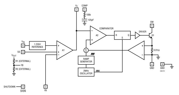
Figure 1. Block Diagram
