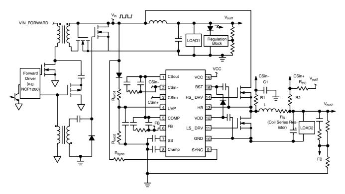
Figure 27. Post-Regulation with CCCV Protection
