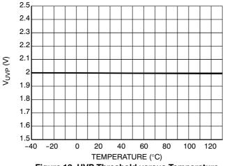
Figure 13. UVP Threshold versus Temperature
