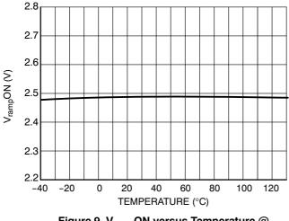
Figure 9.  $V_{ramp}ON$  versus Temperature @  $V_{pin5} = 0.5 V$
