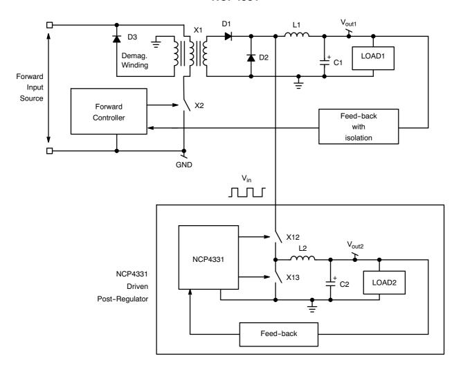
Figure 20. NCP4331 Post-Regulator Associated to a Forward Converter
