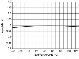
Figure 10.  $V_{ramp}ON$  versus Temperature @  $V_{pin5}$  = 2.0 V
