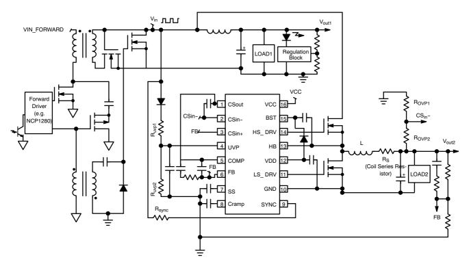
Figure 26. "Basic" Configuration Further Including an Overvoltage Protection (OVP)
