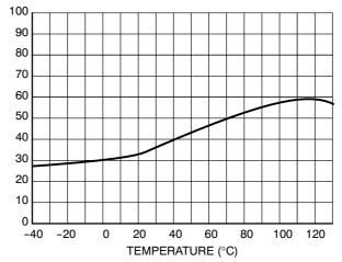
Figure 14. Hysteresis of the UVP Comparator versus Temperature
