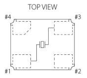
• #1,#3 : Crystal terminal / #2,#4 : Connected to cover (Please connect it with GND.)
