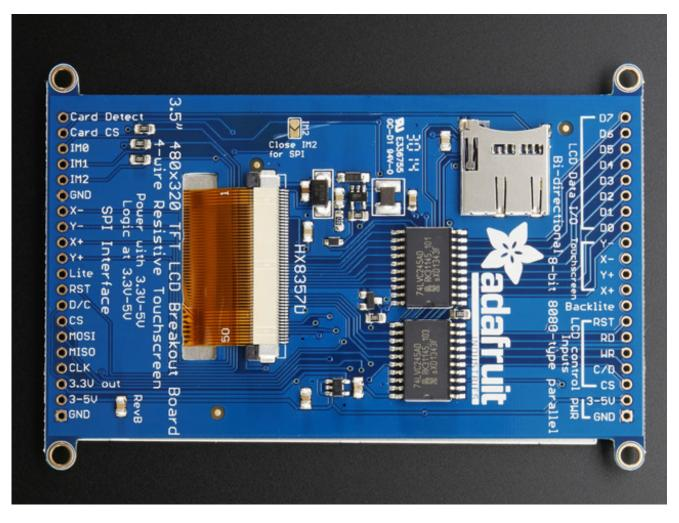
The 3.5" TFT display on this breakout supports many different modes - so many that the display itself has 50 pins. However, we think most people really only use 2 different modes, either "SPI" mode or 8-bit mode. Each 'side' of the display has all the pins required for that mode. You can switch between modes, by rewiring the display, but it cannot be used in two modes at the same time!
