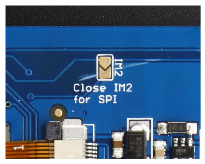
With your soldering iron, melt solder to close the jumper indicated IM2
