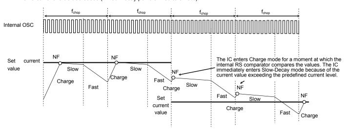
The Charge period starts as the internal oscillator clock starts counting. When the output current reaches the predefined current level, the internal RS comparator detects the predefined current level (NF); as a result, the IC enters Slow-Decay mode.
