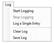
Click **Start Logging** to start the logging function. Each time the program polls the ALS information from the device, it will create a new log entry showing the raw data values, the calculated lux value, the values of various control registers, and the values entered by the user into the text fields near the bottom right corner of the window.
