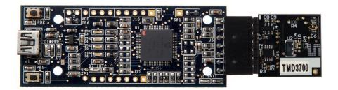
When the USB cable is connected, the green LED should flash indicating that power is being received via the USB interface, and the controller board processor is running. If the green LED does not flash, check the USB cable connections; unplug the USB cable and try again. If the green LED still does not flash, check the PC for USB error messages. See the Resources section at the end of this document for additional assistance.
