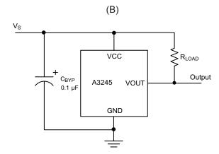
Figure 1: Switching Behavior of Omnipolar Switches. In Panel A, on the horizontal axis, the B+ direction indicates increasing south polarity magnetic field strength, and the B– direction indicates decreasing south polarity field strength (including the case of increasing north polarity). This behavior can be exhibited when using a circuit such as that shown in panel B.
