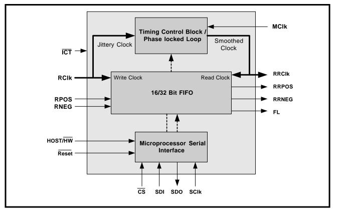
FIGURE 6. ILLUSTRATION OF THE XRT71D00 (CONFIGURED TO OPERATE IN THE "HOST" MODE)
