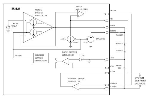
Figure 3A - Output 1 System Set Point Test Circuit
