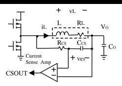
Figure 7 Inductor Current Sensing and Current Sense Amplifier
