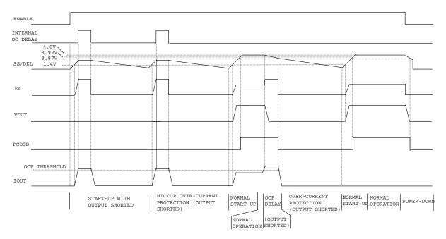
Figure 13 Hiccup over-current waveforms
