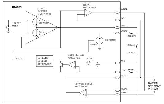
Figure 3B - Output 2 System Set Point Test Circuit
