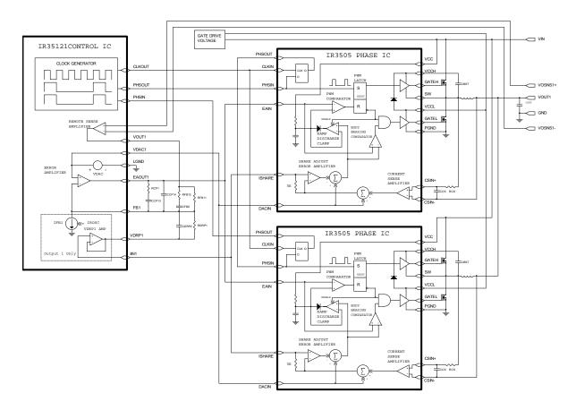
Figure 4 - PWM Block Diagram
