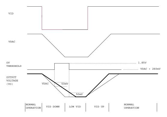
Figure 16 Over-voltage protection during dynamic VID
