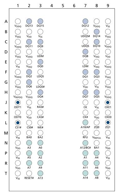
Note: 1. Dark balls (with rings) designate balls that differ from the monolithic versions.
