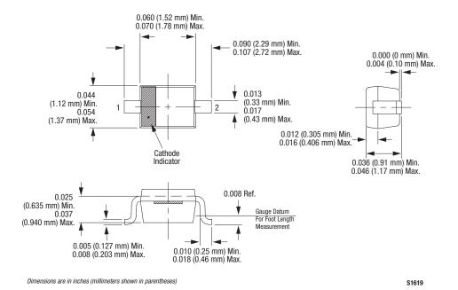
Figure 9. SOD-323 Package Dimension Drawing
