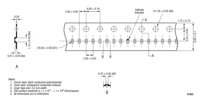
Figure 12. SOD-882 Tape and Reel Dimensions
