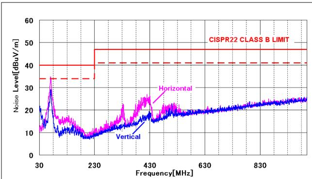
Figure 4: EMI Test Data of MP7752 EVB
