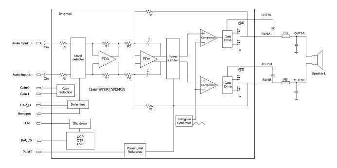
**Functional Block Diagram (only one channel)**
