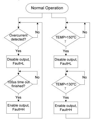
Figure 3: Fault Timing Chart
