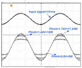
Figure 2. PLIMT Circuit Operation
