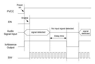
Figure 1b: enable on with audio signal present Adjustable Power Limit
