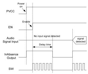
Figure 1a: enable on with no signal detected
