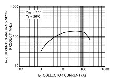
Figure 5. Current Gain Bandwidth Product vs.
