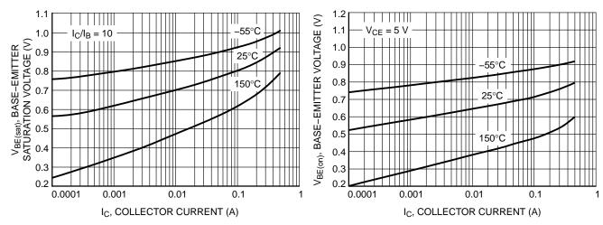
Figure 11. Base Emitter Saturation Voltage vs.
