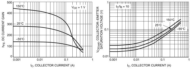
Figure 1. DC Current Gain vs. Collector Current
