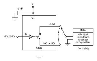
Figure 5. Channel Off/On Capacitance
