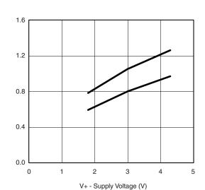
Switching Threshold vs. Supply Voltage
