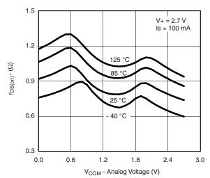
r<sub>ON</sub> vs. Analog Voltage and Temperature
