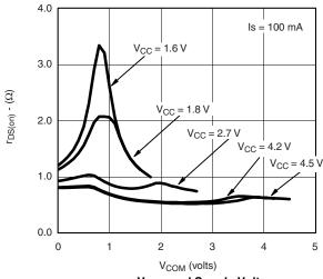
$r_{\mbox{\scriptsize ON}}$  vs.  $V_{\mbox{\scriptsize COM}}$  and Supply Voltage
