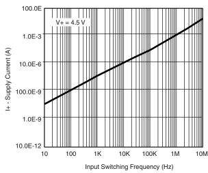
**Supply Current vs. Input Switching Frequency**
