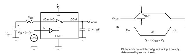
Figure 3. Charge Injection
