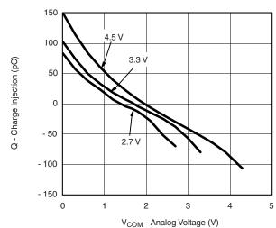
Charge Injection vs. Analog Voltage
