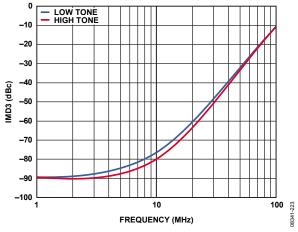
Figure 22. IMD3 vs. Frequency
