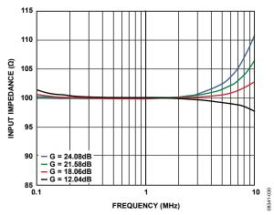
Figure 11. Input Impedance R<sub>IN</sub> vs. Frequency, 100  $\Omega$  Active Termination
