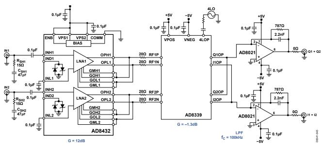
Figure 71. Schematic of the AD8432 (G = 12.04 dB) and AD8339 Application for Ultrasound Beamforming
