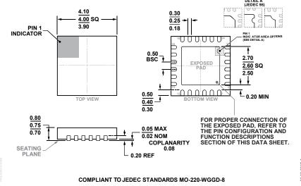
Figure 81. 24-Lead Lead Frame Chip Scale Package [LFCSP] 4 mm × 4 mmand 0.75 mm Package Height (CP-24-15) Dimensions shown in millimeters
