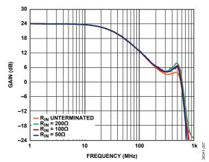
Figure 7. Small Signal Frequency Response vs.  $R_{IN}$ , G = 24.08 dB
