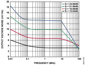
Figure 21. Output Voltage Noise vs. Frequency
