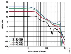
Figure 9. Differential Gain vs. Frequency,  $V_{OUT} = 2 V p$ -p,  $R_{IN} = 50 \Omega$
