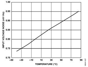
Figure 18. Input Voltage Noise vs. Temperature
