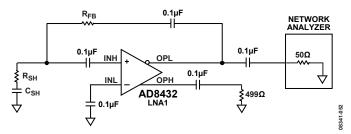
Figure 63. Output Impedance vs. Frequency Measurements
