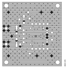
Figure 78. AD8432-EVALZ Ground Plane Copper
