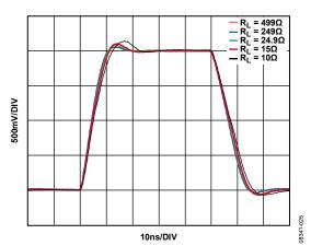
Figure 50. Large Signal Transient Response vs. Resistive Load ( $R_L$ ),  $G = 24.08 \, dB$
