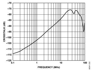
Figure 36. Channel Crosstalk vs. Frequency
