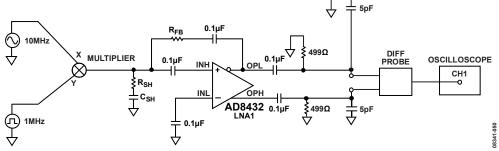
Figure 61. Overdrive Recovery Measurements
