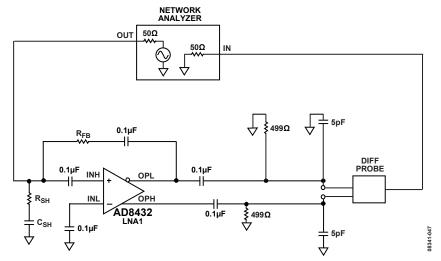
Figure 59. Frequency Response Measurements
