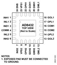
Figure 2. Pin Configuration
