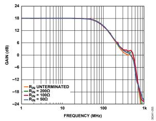
Figure 5. Small Signal Frequency Response vs.  $R_{IN}$ , G = 18.06 dB
