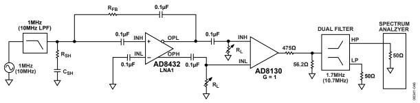
Figure 57. Harmonic Distortion vs. Resistive Load (R<sub>L</sub>) Measurements
