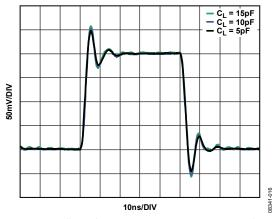
Figure 41. Small Signal Transient Response vs. Capacitive Load ( $C_L$ ),  $G = 12.04 \, dB$
