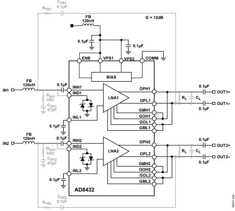
Figure 69. Typical AD8432 Setup, G = 12.04 dB
