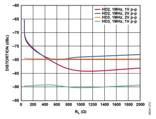
Figure 33. Harmonic Distortion at 1 MHz vs. Resistive Load ( $R_L$ ),  $G=24.08\ dB$
