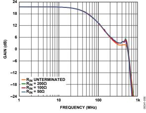
Figure 6. Small Signal Frequency Response vs.  $R_{IN}$ , G = 21.58 dB
