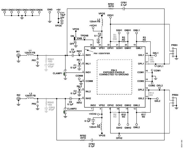
Figure 80. AD8436-EVALZ Schematic
