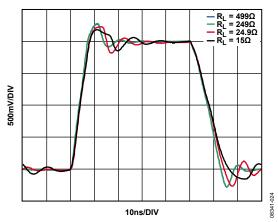
Figure 49. Large Signal Transient Response vs. Resistive Load ( $R_L$ ),  $G = 12.04 \, dB$
