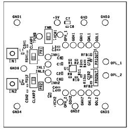
Figure 74. Evaluation Board Assembly
