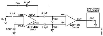
Figure 64. Noise Figure Measurements
