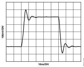
Figure 40. Small Signal Transient Response,  $G = 12.04 \, dB$
