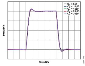
Figure 42. Small Signal Transient Response vs. Capacitive Load (C<sub>L</sub>), G = 24.08 dB
