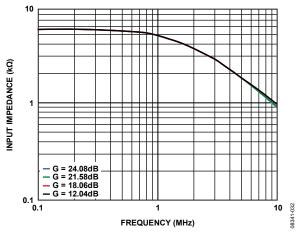
Figure 13. Input Impedance  $R_{IN}$  vs. Frequency, Unterminated
