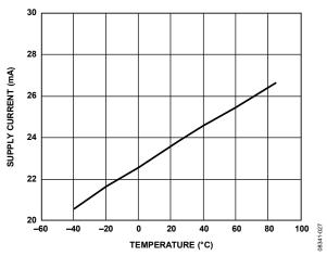
Figure 53. Supply Current vs. Temperature
