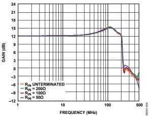
Figure 4. Small Signal Frequency Response vs.  $R_{IN}$ , G = 12.04 dB
