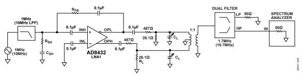
Figure 58. Harmonic Distortion vs. Capacitive Load (C<sub>L</sub>) Measurements
