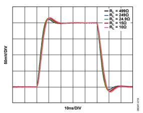
Figure 44. Small Signal Transient Response vs. Resistive Load ( $R_L$ ),  $G = 24.08 \, dB$
