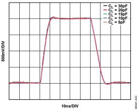
Figure 48. Large Signal Transient Response vs. Capacitive Load ( $C_L$ ), G = 24.08 dB
