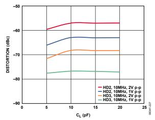
Figure 26. Harmonic Distortion at 10 MHz vs. Capacitive Load (C<sub>L</sub>), G = 12.04 dB
