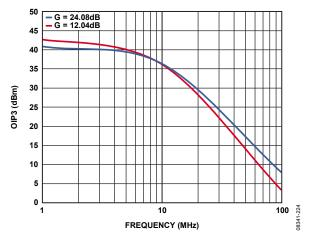
Figure 23. Output Third-Order Intercept vs. Frequency
