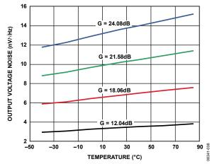
Figure 19. Output Voltage Noise vs. Temperature
