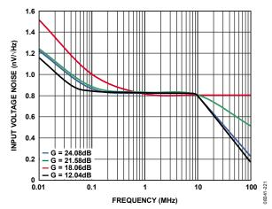
Figure 20. Input Voltage Noise vs. Frequency
