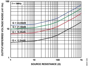
Figure 17. Output-Referred Voltage Noise vs. Source Resistance (Rs)
