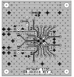
Figure 75. AD8432 Primary Side Copper
