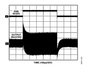
Figure 55. Small Signal Enable Response
