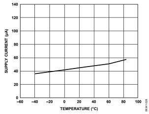
Figure 54. Supply Current vs. Temperature in Disable Mode
