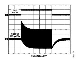
Figure 56. Large Signal Enable Response
