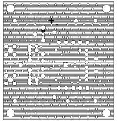
Figure 77. AD8432-EVALZ Power Plane Copper
