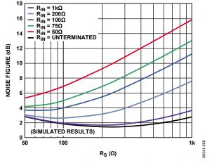
Figure 68. Noise Figure vs. R<sub>5</sub> for Various Values of R<sub>IN</sub>, Actively Matched
