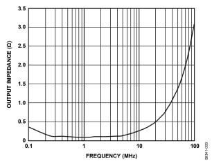
Figure 14. Output Impedance vs. Frequency
