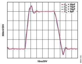
Figure 47. Large Signal Transient Response vs. Capacitive Load ( $C_L$ ),  $G = 12.04 \, dB$
