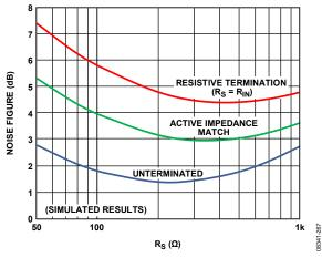
Figure 67. Noise Figure vs. R<sub>S</sub> for Resistive, Active Match, and Unterminated Inputs
