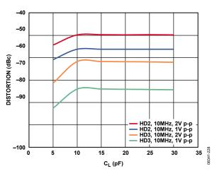
Figure 28. Harmonic Distortion at 10 MHz vs. Capacitive Load (C<sub>L</sub>), G = 24.08 dB
