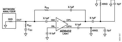
Figure 62. Input Impedance vs. Frequency Measurements
