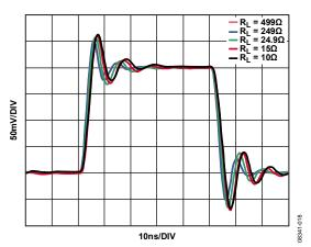
Figure 43. Small Signal Transient Response vs. Resistive Load ( $R_L$ ),  $G = 12.04 \, dB$
