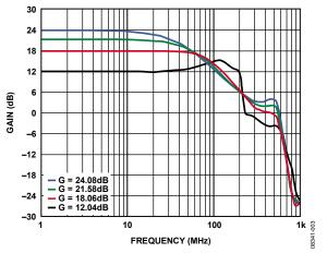
Figure 3. Small Signal Differential Gain vs. Frequency, R<sub>IN</sub> Unterminated
