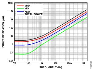
Figure 45. Power Dissipation vs. Throughput, VIO = 1.8 V,  $V_{REF} = 5 \text{ V}$
