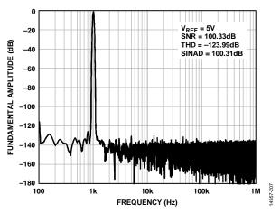
Figure 12. 1 kHz, -0.5 dBFS Input Tone FFT, Wide View,  $V_{REF} = 5 V$
