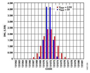
Figure 14. Histogram of a DC Input at Code Transition,  $V_{REF} = 2.5 V$ , 5 V
