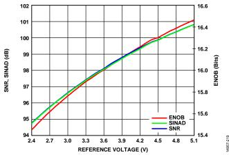
Figure 17. SNR, SINAD, and ENOB vs. Reference Voltage
