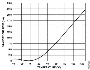
Figure 27. Standby Current vs. Temperature
