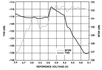
Figure 20. THD and SFDR vs. Reference Voltage
