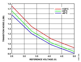
Figure 10. Transition Noise vs. Reference Voltage
