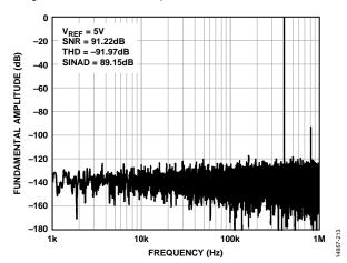
Figure 16. 400 kHz, -0.5 dBFS Input Tone FFT, Wide View
