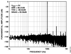
Figure 13. 100 kHz, -0.5 dBFS Input Tone FFT, Wide View
