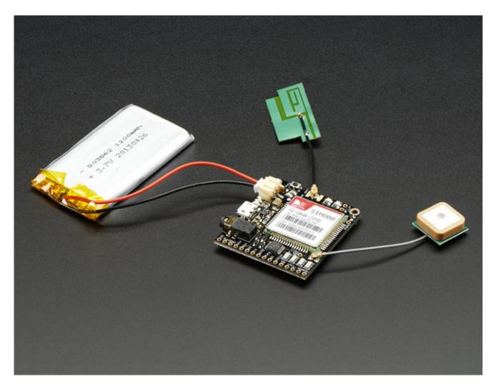
Check polarity for the battery!
