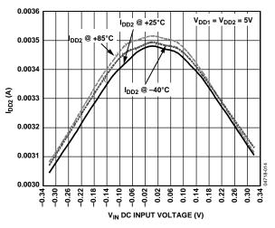
Figure 15. IDD2 vs. VIN at Various Temperatures
