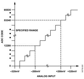
Figure 21. Filtered and Decimated 16-Bit Transfer Characteristic
