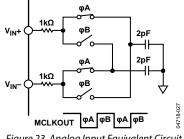
Figure 23. Analog Input Equivalent Circuit
