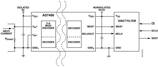
Figure 22. Typical Application Circuit
