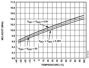
Figure 19. MCLKOUT vs. Temperature for Various Supplies
