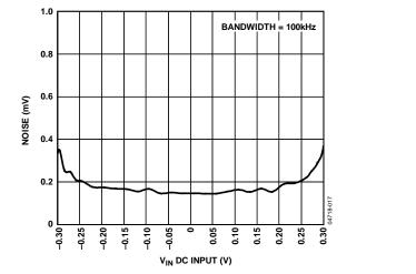
Figure 18. RMS Noise Voltage vs. V<sub>IN</sub> DC Input
