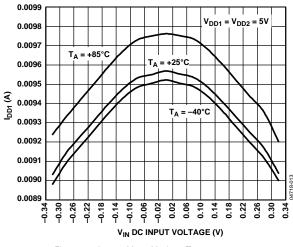
Figure 14. IDD1 vs. VIN at Various Temperatures
