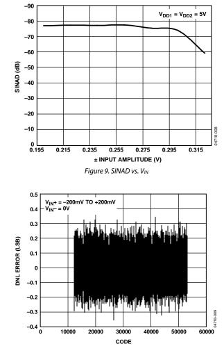
Figure 10. Typical DNL, ±200 mV Range (Using Sinc<sup>3</sup> Filter, 256 Decimation Rate)
