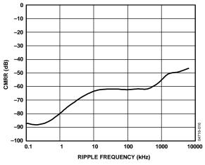
Figure 17. CMRR vs. Common-Mode Ripple Frequency
