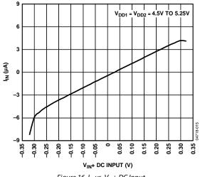
Figure 16. IIN vs. VIN+ DC Input
