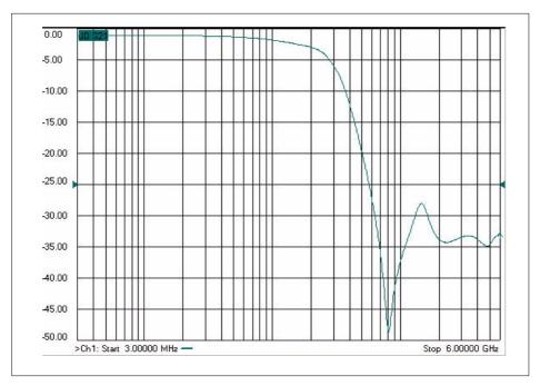
Figure 1. Typical Filter Insertion Loss (CM1693)
