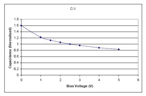
Figure 2. Filter Capacitance vs. Input Voltage (Normalized to Capacitance at 0 VDC and 25°C)
